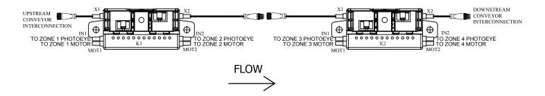
There are two types of accumulation release: Singulation release and Slug release. Singulation release allows one product to be released at a time after the downstream zone has cleared. Slug release allows a predetermined amount of product to be released at one time after the downstream zone has cleared. Slug release is typically used in Palletizing or Machine loading conditions. The type of release to be used is usually determined at design time.
